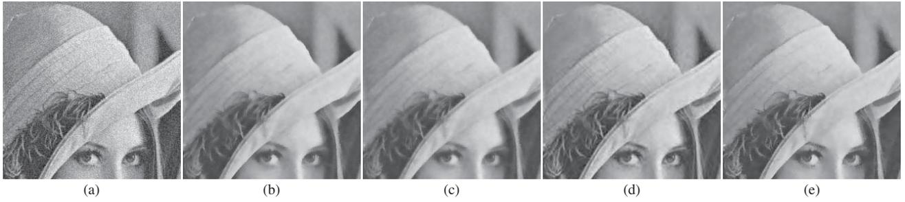
Fig. 1. Results for part of the  $512 \times 512$  *Lena* test image corrupted with additive white noise of  $\sigma = 15$ . (a) Noisy image: PSNR = 25.31 dB. (b) FBF denoising result: PSNR = 30.96 dB. (c) GIF denoising result: PSNR = 30.87 dB. (d) SURE-LET denoising result: PSNR = 32.56 dB. (e) LLSURE denoising result: PSNR = 31.93 dB.
