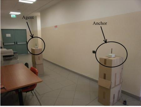
Fig. 3. Adopted experimental setup for a LOS link; the employed radio devices are located on the top of two paper boxes.
