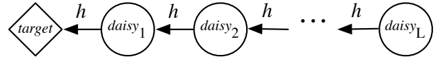
Fig. 5. Given daisy_i it is easy to verify the freshness of the blacklist by applying h i times to obtain target . Only the NM can compute the next daisy_{i+1} in the chain.
